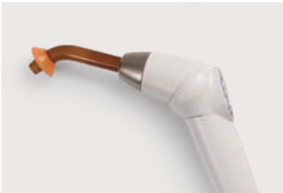
T-LED The curing light can be used as a direct version or 120° angled version. With a high-power LED up to a maximum of 2,200mW/cm² and a 430 to 490nm emission band, the T-LED lamp offers 6 pre-set programmes and a sterilisable optical guide.
